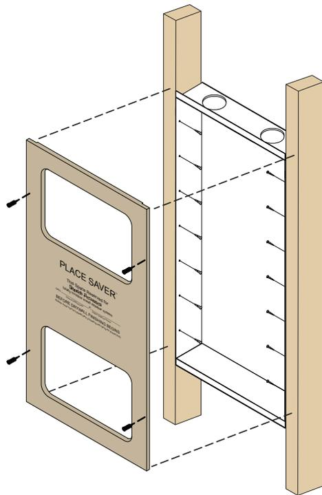
The PlaceSaver™ mounts over back box to ensure proper rough opening
