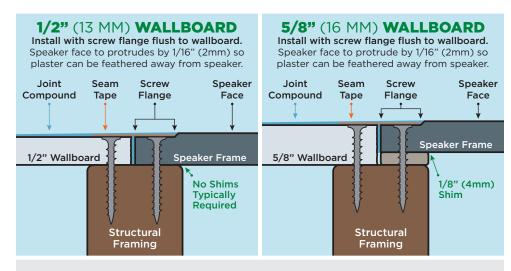
Note: The typical installations shown above are provided as guidelines. For your installation, the number and thickness of shims needed may differ due to variances in wallboard material and other construction variables.
